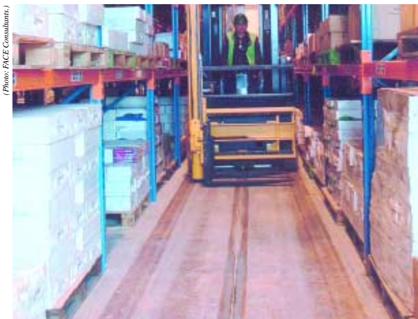
Figure 1: Mechanical Handling Equipment (MHE) uses fixed paths in very narrow aisles.
