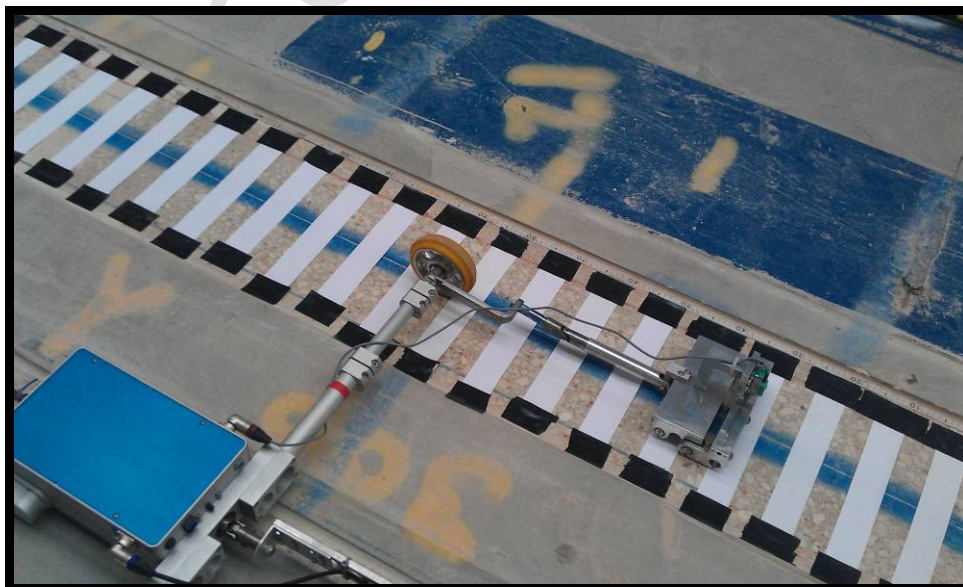
Fig. 6 – Re-run of the Face Digital profileograph with the VDMA Fx meter
