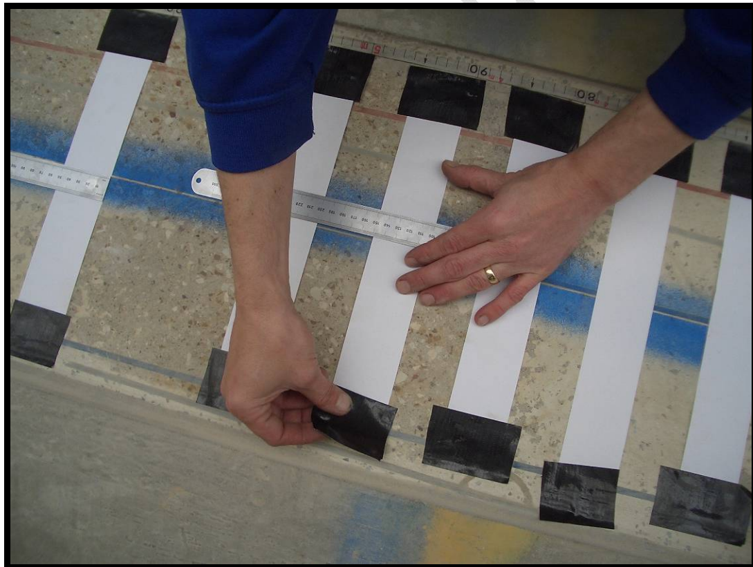
Fig. 4 – Placing the 50mm strips at 50mm spacing.
